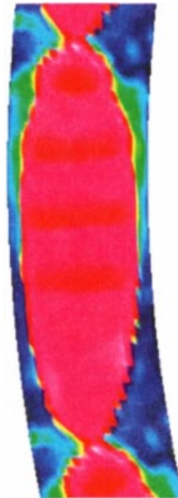
Fig. 6 Total velocity contours between nozzle exit and blade leading edge
